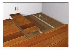
Measure the shower drain base position on the floor and mark this onto the relevant piece of plywood. Using a jigsaw cut a hole in the plywood so the shower drain base and shower drain connector will be exposed through the new floor. Please note that the hole should be no bigger than 180x180mm.
